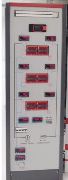
**Figure 7.** An 18-kVA 3-phase cabinet has been designed to demonstrate a concrete power routing example.
