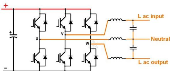
**Figure 3.** ECI converters enable a 0-ms transfer time between AC and DC power input thanks to their AC/DC/AC converter and common DC energy buffer (left).
