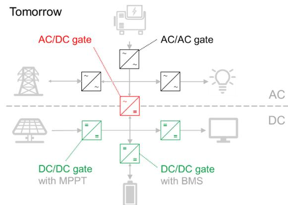
**Figure 1.** By comparison to today's AC-based infrastructures relying on unidirectional converters, tomorrow's electricity management involves smart energy gates consisting of bidirectional converters.
